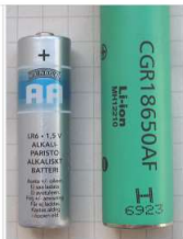
An 18650 size lithium ion battery, with an alkaline AA for scale. 18650 are used for example in notebooks or Tesla Model S
